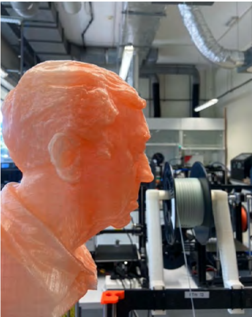
3D print of the head of Prof. Bogdan Marciniec, the creator and first director of the Centre. The printout was made of biomaterial and was based on a laser scan
